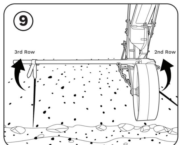
Stop at the end of the first run and place the marker back in its holder in the vertical position. The marker will have left a trail to be followed for the next seeding row (2nd Row). Now place the marker on the opposite side (on your left) and push the seeder along the track made by the marker on your first run (2nd Row).
