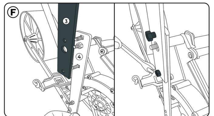
Align the holes of item 3 (Handle Section) with the bolts protruding from item 4 (main body frame). Place item 3 (handle section) onto item 4 (main body frame) and tighten the highlighted nuts.
