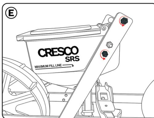
Remove the highlighted nuts from item 4 (main body frame). Remove the same nuts on the reverse side.
