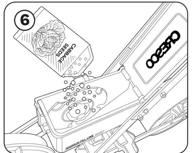
Empty the seeds into the hopper but make sure you do not exceed the maximum fill line. Overfilling can result in over application which will damage your yield.
