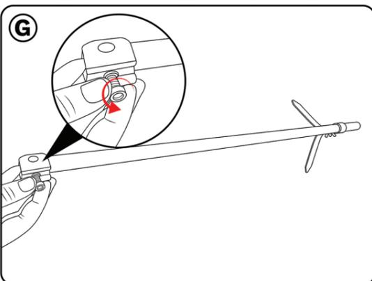
Take item 5 (row marker arm) and remove the nut located at the bottom end.
