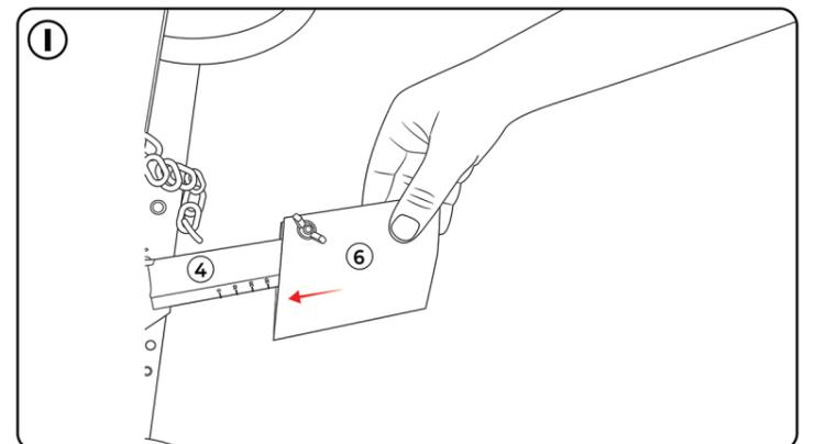
Take item 6 (Depth setting blade) and loosen the wing nut slightly. Slide item 6 (Depth setting blade) onto the depth marker protruding from the bottom of item 4 (main body frame).
