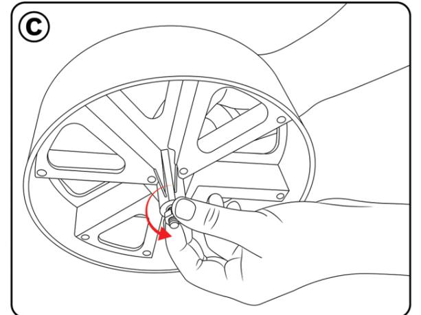
Remove the long bolt located through the middle of item 2 (Rear wheel).
